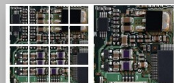
Real-time stitching can generate mosaic images while moving the stage
